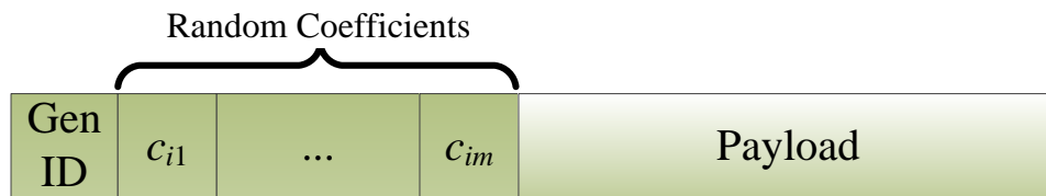
Figure 2.7 Network Coding packet format
